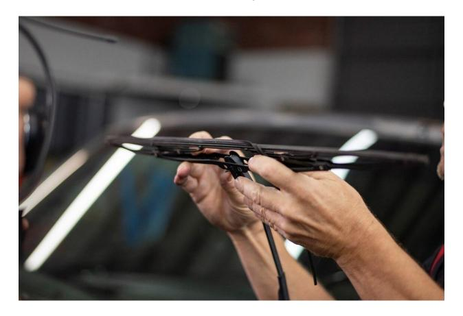
Beam blades, also known as frameless wiper blades, have recently gained popularity. Beam blades are longer and thinner than traditional wiper blades. In place of the typical metal frame, they use a single, continuous piece of rubber or silicone to wipe the windscreen. At <u>Leicester Motor Spares</u>, customers can choose from a choice of frameless wiper blades, each of which offers enhanced wiping effectiveness in addition to increased longevity.
